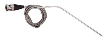
GF 3T Pt1000 – The Class B insertion sensor is suitable for use in gases, liquids and soft plastic materials. The stainless steel tube of the insertion sensor is designed for permanent contact with foods. The 1-metre-long glass fibre insulated cable is encased with a stainless steel braided jacket, heatresistant to 400 °C and equipped with a BNC plug connector. Ideal for long-term measurements in ovens or grills.
