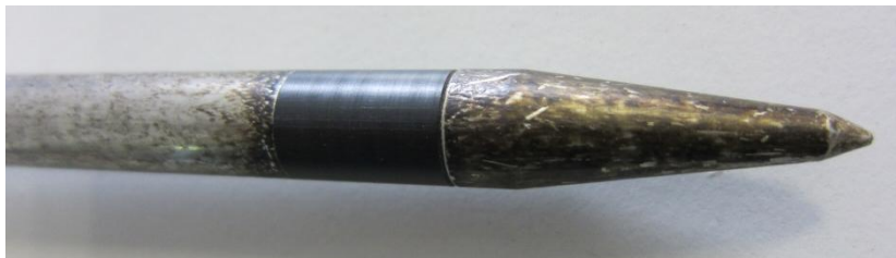
Soiled probe -> wrong measuring!
